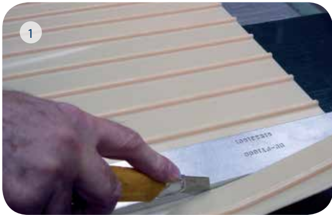
Cut the belt using the Cutting Bar to the required length.
