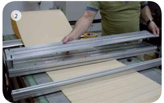
Select the appropriate adapter for the belt type to be welded. Position the Adapter onto the pliers when the groove of the electrode is facing up.
