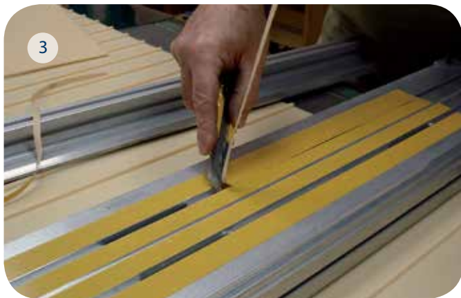
Apply Double-side Tape on the Adapter surface and trim the unnecessary tape from the grooves. At this stage do not remove the protective paper.
