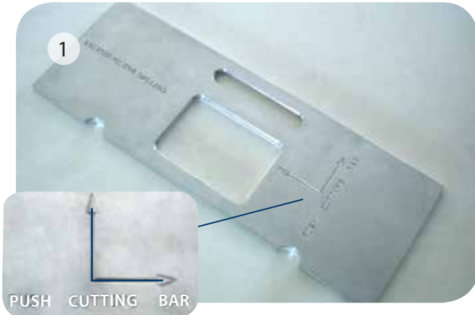
1. The cutting bar is marked with positioning arrows as per photo 2
