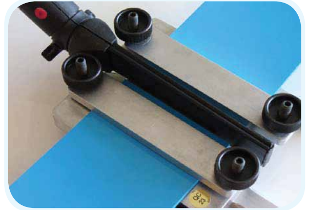
Welding narrow flat belts with Pliers P-200
