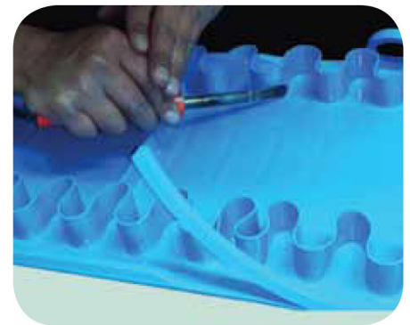
Sidewalls and Guides endless welding
